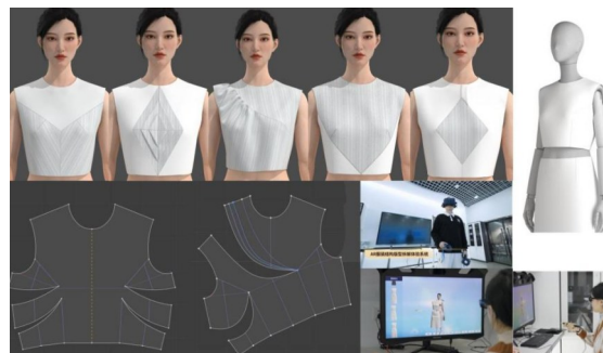
Figure 8 Holographic AR Garment Structure Reverse Disassembly System and 3D Digital Virtual Simulation Case of Garment Structures
